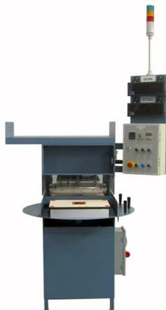
These machines feature quick-change sealing fixtures and quick change relieved face plates for fast tooling changeover. This has given the client the opportunity to operate lean manufacturing and still meet customer requirements. Multiple machines can run the same product if the volume is high or the machines can all be running different SKU's to provide a continuous output of over 30 different packages.
