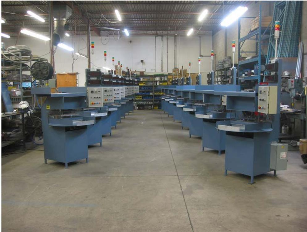
No, this is not a mirrored photo. This was one of three groups of machines ordered by a major consumer goods manufacturer. These MR2-1418 machines have production goal displays and light towers that allow supervisors to observe operation at a glance. These special machines included a shelf on top of the machine for packaging materials that included a sensor to double check that the operator has picked all of the components for each package.
