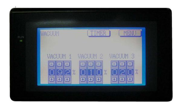
A typical set-up might be Stage 1-a short time and high vacuum speed to evacuate air from under the film quickly, Stage 2 - a longer time and low vacuum speed to reduce webbing and keep film from rupturing around complex parts and finally Stage 3 – a relatively long time and higher vacuum to pull film tightly to the board and provide cooling. Any stage may be skipped by entering zero time.
