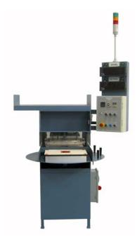
These machines feature quick-change sealing fixtures and quick change relieved face plates for fast tooling changeover. This has given the client the opportunity to operate lean manufacturing and still meet customer requirements. Multiple machines can run the same product if the volume is high or the machines can all be running different SKU's to provide a continuous output of over 30 different packages.
