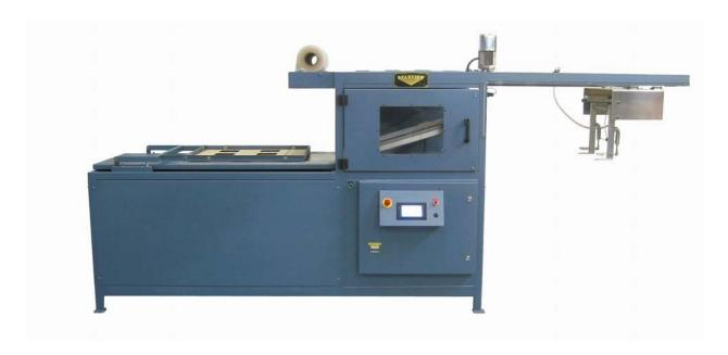
Starview's ASP-2430 Skin Packaging Machine with automatic in-feed, moving template loader and automatic out-feed.
