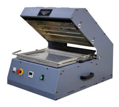
We have updated the design of the MSP-1218 to incorporate the features used on the MSP-1824 released last year. The new film clamping frame with upper and lower gas filled cylinders makes it much easier for the operator to raise and lower. This machine still uses readily available standard 20" wide film and nominal 12" x 18" skin boards.
