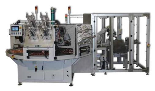
Starview recently completed the above machine for one of our European Pharmaceutical customers. It is a flexible machine designed to produce wallet packs. The primary component of the system is a FAB/PH6-1824 automatic rotary heat sealing machine. The rotary machine feeds the cards and the capsule packages. There are options to fold the cards by hand or with the automatic folder. The press is designed for either heat seal or for the Ecobliss patented cold seal.
