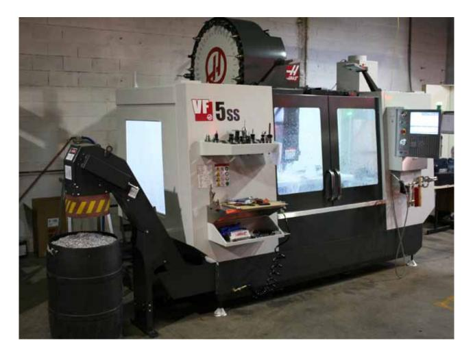
Starview just added a third new CNC vertical machining center to increase capacity is our machining department. This brand new Haas VF5SS gives us additional tooling capability as well as the ability to process large machine components. It is 50" x 26" in the X and Y axis with 25" under the spindle. A 40 +1 position tool changer gives us very fast set-up.
