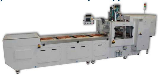
Starview recently completed the above inline sealing machine for the production of pharmaceutical wallet packs. The package materials are hand loaded. The sealing press is universal and can be used for heat sealing or a cold seal process that uses encapsulated adhesive. Finished packages are automatically unloaded from the machine and placed on a conveyor running at 90 degrees to the machine direction.
