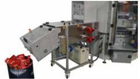
UNLOAD STATION WITH PACKAGE SLITT
